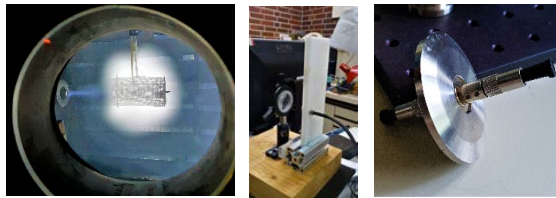
Fig. 1: Optical measurements through (a) a window; (b) lens projection on a screen, (c) a fiber optic adaptor.
